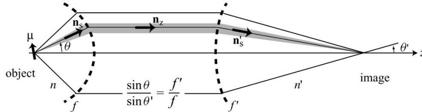
Figure 1: Configuration used for the calculation of the point-spread function. The source is an arbitrarily oriented electric dipole with moment  $\mu$ . The dipole radiation is collected with a high-NA aplanatic objective lens and focused by a second lens on the image plane at  $z = 0$ .
