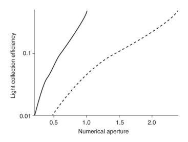
The collection efficiency is the fraction of photons emitted into a solid angle  $\Omega$  given by  $\frac{\Omega}{4\pi}$ . The maximum angle at which the emitted photons to be collected is known as  $\theta$ . The fraction F which is collected in this case will be:
