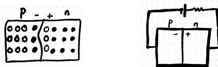
In a typical junction (e.g. pn-junction) the field developed in the depletion region is enough to stop carrier diffusion. The associated barrier voltage is also called built-in voltage as shown in figure below. The reverse bias widened the depletion region and the field becomes stronger.
