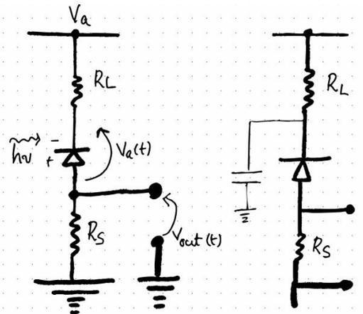
The bias voltage is applied through a large ballast resistor  $R_L$ . A small resistor  $R_S$  is connected to the other terminal for observing the current pulse. The avalanche current discharges the total capacitance at the diode terminal. The voltage across the diode decreases toward  $V_{BD}$  and the avalanche decreases. As the voltage decreases to  $V_{BD}$ , the rate of avalanche decreases. All the avalanche current flows through  $R_L$  and is reduced to,  $\frac{V_a - V_{BD}}{R_L}$ .
