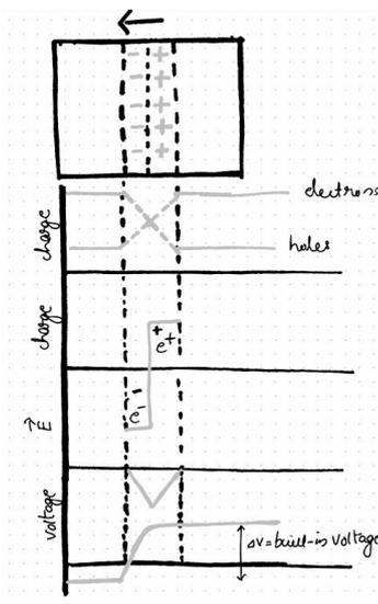
Figure 1: Built-in voltage due to pn-junction
