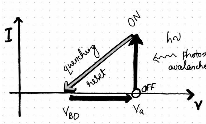
Photon assisted carrier generation trigger the avalanche effect and switch the device to ON state. The device stays ON until the avalanche is quenched by an external circuit (quenching circuit) and reset for the other photon event detection.
